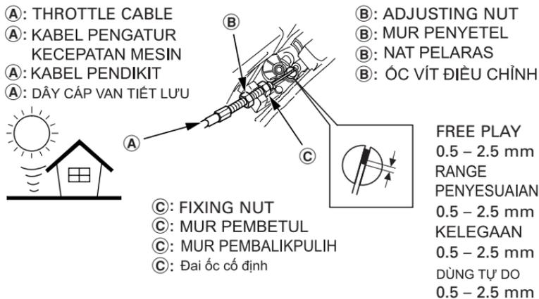
1. Check the throttle cable free play at the tip of the cable. Adjust the free play with adjusting nut and fixing nut, if necessary.
