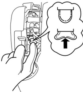
3. Remove the oil filler cap and drain the oil.
