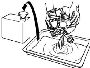
2. Press the priming pump several times and drain the fuel from the fuel tank again.
