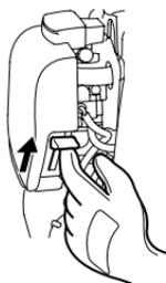
3. Press the priming pump several times until fuel stays in the priming pump.
