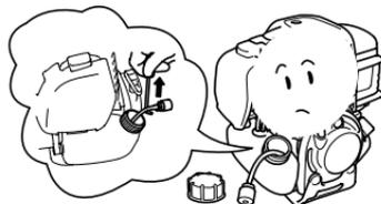
4. Remove water and dirt stood in the fuel tank by rinsing its inside.
