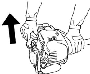
5. Turn the choke lever to the open position.
