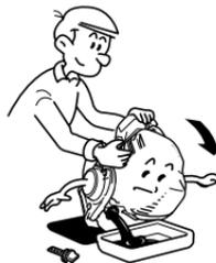
2. Drain the oil by tilting the engine.
