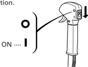
2. Turn the choke lever to the close position, if necessary.
