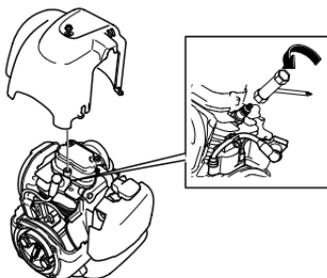
Clean, gap or replace the spark plug.
