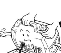
2. Refill with the motor oil (see page 3) and check the oil level.
