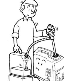
2. Loosen the drain screw and drain the fuel.
